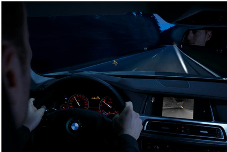
The night-vision system produced by Autoliv in Goleta highlighted in BMW promotional materials. The automakers cars alert drivers of nearby pedestrians and animals in four ways: an infrared display, the instrument panel, the heads-up display and a spotlight. (Photo courtesy Autoliv)
