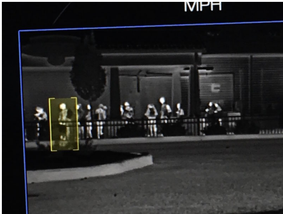
THE NIGHT VISION SYSTEM FRAMES PEOPLE WHO ARE WALKING SO YOU CAN SEE THEM. PHOTO: SCOTTY REISS FOR SHEBUYSKARS
